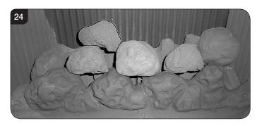
5.18 Place the rear right medium coal in the recess behind the front row of coals resting on the rear pane, see Diagram 25.
