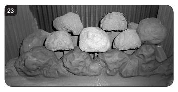
8.19 Place the right hand small coal in the recess between the flame baffle and the front coal, see Diagram 24.
