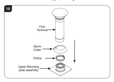
4a.11 Tighten the flue pipe Clamp to secure the Flue Terminal in place, see Diagram 17.
