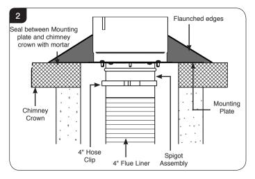
3a.3 Secure the Mounting plate to the chimney crown with four screws and flaunch the edges of the plate with additional mortar to create a smooth run off that ensures the rain water will not collect around the spigot.
