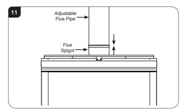
3d.2 Extend the adjustable flue pipe to connect the appliance to the lower mounting plate assembly. The minimum usable length of the adjustable flue pipe section is 300mm, the maximum is 490mm.
