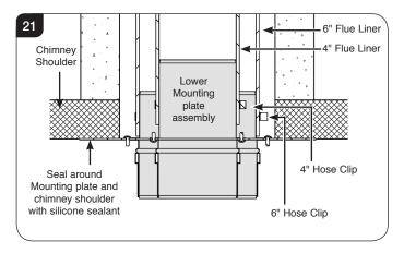
4b.8 The bottom of the chimney may require a larger register plate. This can be achieved by cutting a 175mm (7") diameter hole in the register plate and securely sealing the lower Mounting Plate Assembly onto the register plate, see Diagram 22.
