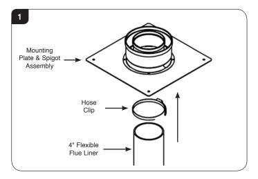
Tighten the Hose Clip so that the liner is held securely to the spigot.
