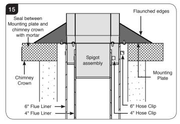
4a.9 Secure the Mounting Plate to the chimney crown with four screws and flaunch the edges of the plate with additional mortar to create a smooth run off that ensures the rain water will not collect around the spigot.
