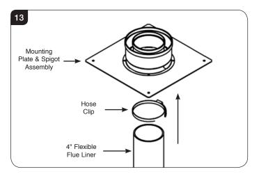
4a.3 Tighten the 4" Hose Clip so that the liner is held securely to the spigot.
