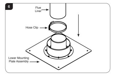
Tighten the 4" Hose Clip so that the liner is held securely to the spigot.
