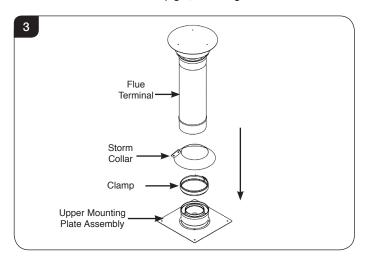
3a.5 Tighten the flue pipe Clamp to secure the Flue Terminal in place, see Diagram 4.
