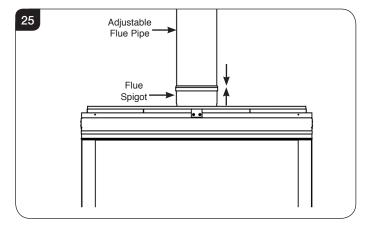
4d.2 Extend the adjustable flue pipe to connect the appliance to the lower mounting plate assembly. The minimum usable length of the adjustable flue pipe section is 300mm, the maximum is 490mm.
