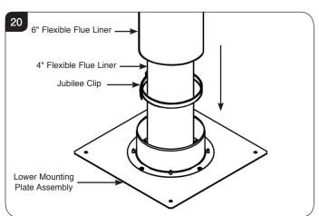
4b.6 Tighten the 6" Hose Clip so that the liner is held securely to the spigot.
