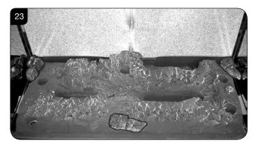
8.19 Place Log D on the left hand side of the burner. There is a hole on the underside of Log D which fits over the raised stud on the left of the burner. The back of the log should rest flat against the back panel, see Diagram 24.
