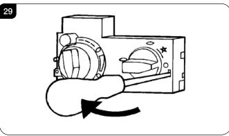
7.4 Disconnect the other end of the ignition lead from the valve body noting the route of the ignition lead.
