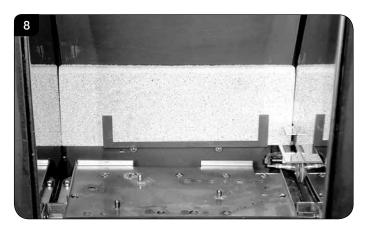
4.6 Replace all parts in reverse order ensuring the cutouts in the rear of the lower panel fit over the screws on the back of the firebox, see Diagram 9.
