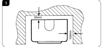
5.4 In a non-combustible recess be careful to allow enough clearance at the sides and rear of the appliance to perform spillage tests and reach the controls.
