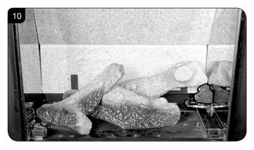
8.6 Place the foot of Log C into the rear left hand corner. The long flat edge rests against the side of the firebox and the log touches the back panel. The top of the log rests on Log E, see Diagram 11.
