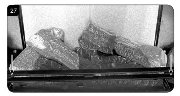
8.23 Place Log A across Log C. There is a hole on the underside of Log A which fits over the raised stud on Log C to secure in place. The small cut out on the left side of the log rests onto the log guard, see Diagram 28.
