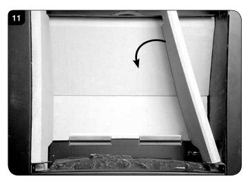
4.10 To remove the Right Hand liner first tilt inwards towards the centre of the firebox before lifting up and pulling out through the front of the firebox, see Diagram 11.
