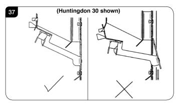
12.10 Replace the metal panel. There are spacers on the top edge to ensure the correct distance from the baffle. These interlock with the rear of the baffle, see Diagram 38.
