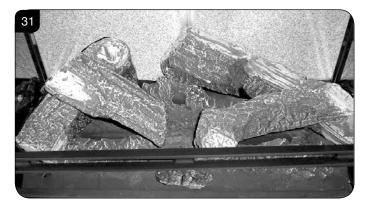
7.24 Once the logs are in place use some of the Embaglow wire wool provided and cover the ports in the burner tray with a liberal amount of fibres, in the highlighted areas shown in Diagram 32.
