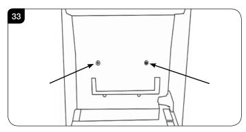
12.3 Remove the two screws securing the metal panel at the rear of the firebox, see Diagram 34.
